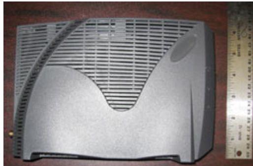
This is the router that plugs into the Receiver and into your computer or Hub
